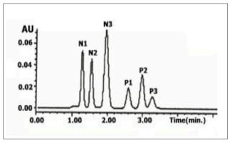
Mobile phase: 60:40 acetonitrile/DI water + 0.5% formic acid Samples: Proprietary drugs: N1 - N3 nucleoside analogs, P1 - P3 other more hydrophobic proprietary compounds with polar functional groups
