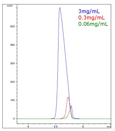
Injection volume is important and should be considered in the method as well.
