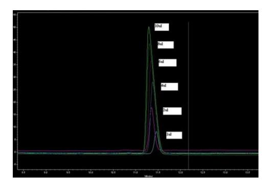
To get sharp, symmetrical peaks simply inject less amount when working in ANP.
