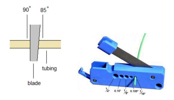
**In order to get the best cut,** you need to use the hole that is designated for the correct diameter tubing. The tubing cutter is equipped with holes to accommodate five different tubing ODs: 1/4", 0.15", 1/8", 0.105", and 1/16". The tubing should fit snugly in the appropriate hole. In the picture above, the indicating arrow is not shown and is on the opposite side of the cutter displayed.
