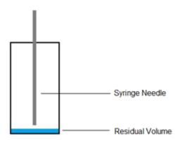
Unlike other vials, the  $AQ^{\text{TM}}$  and  $RSA^{\text{TM}}$  brand Vials have a specification for bottom height. This specific tolerance of the bottom height allows you to bring the needle down to the lowest position necessary.
