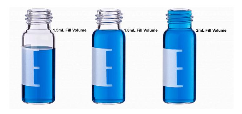
As shown above the Volume of a 12x32mm screw vial when completely filled, it will contain approximately 2mL. This volume for Autosampler filling is called a total fill volume. When other volume designations are used, this is called a nominal volume.
