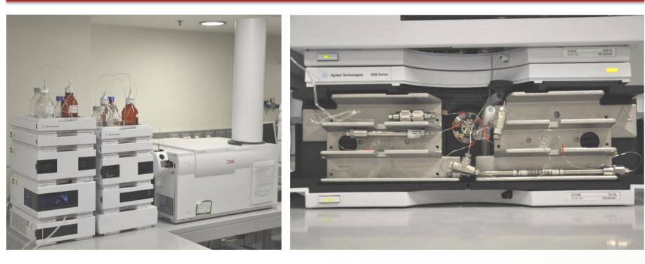
LC: Agilent 1200 series comprising of two degassers, two binary pumps, an auto sampler and a column compartment containing a 10-port 2-position value (a minimum of 8 ports are required) ANP column: Cogent Diamond Hydride 2.1 mm  $\times$  100 mm, 4µm particle size (MicroSolv Technology, Australia).
