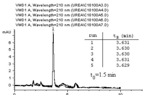
Figure above show 5 consecutive runs using 100% water mobile phase without any loss of precision.
