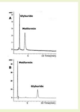
**Notes:** Elution order was confirmed by LC-MS, APCI+, with single ion monitoring Metformin (m/z 130) and Glyburide (m/z 369).
