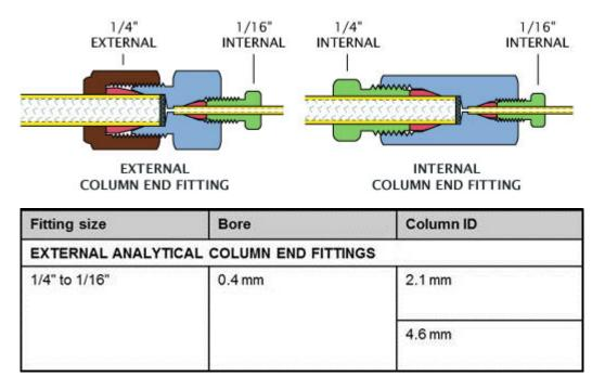
The use of Direct Adaptive Di-Ad<sup>™</sup> column connectors are recommended because they do not permanently lock into place on the connecting tubing, avoiding potential dead volume connection problems. A good connection can therefore be made every time, avoiding the issues that can occur when using a ferrule that gets swaged on the tubing.
