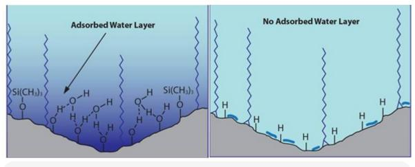
HILIC Phases have a Water Shell and Cogent TYPE-C Silica Does Not
