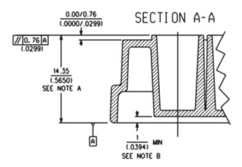
Mechanical Drawings Defining Height Of A Typical Microplate
