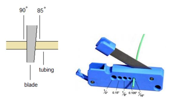
**In order to get the best cut,** you need to use the hole that is designated for the correct diameter tubing. The tubing cutter is equipped with holes to accommodate five different tubing ODs: 1/4<sup>"</sup>, 0.15<sup>"</sup>, 1/8<sup>"</sup>, 0.105<sup>"</sup>, and 1/16<sup>"</sup>. The tubing should fit snugly in the appropriate hole. In the picture above, the indicating arrow is not shown and is on the opposite side of the cutter displayed.
