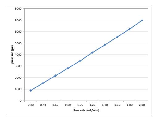
**Column:** Cogent Diamond Hydride<sup>™</sup>, 2.2um 120A, 2.1 x 50mm, cat# 70200-05P-2 **Flow Rate:** 0.2-2.0 mL / minute
