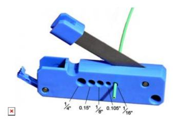
**In order to get the best cut,** you need to use the hole that is designated for the correct diameter tubing. The tubing cutter is equipped with holes to accommodate five different tubing ODs: 1/4", 0.15", 1/8", 0.105", and 1/16". The tubing should fit snugly in the appropriate hole. In the picture above, the indicating arrow is not shown and is on the opposite side of the cutter displayed.
