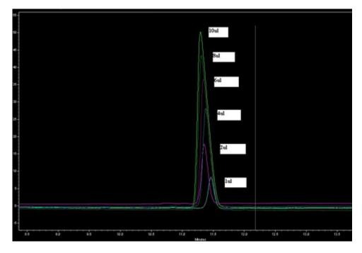
To get sharp, symmetrical peaks simply inject less amount when working in ANP.
